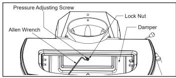
Figure 3.2 - Adjust the damper with the Allen wrench.
