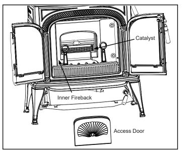
Figure 3.7 - Inspect the catalytic combustor.
