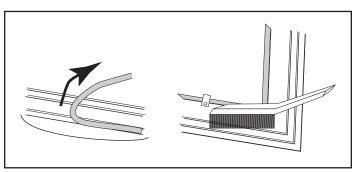
Figure 3.4 - Remove gasket then clean channel with wire brush.
