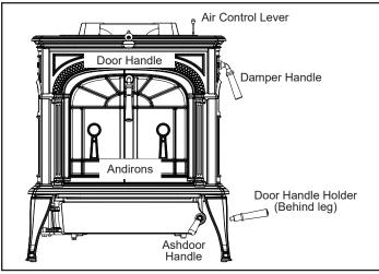
Figure 2.1 - The Intrepid FlexBurn<sup>®</sup> controls are conveniently located and easy to operate.
