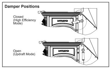
Figure 2.3 - The damper is either open or closed. There are no intermediate positions.
